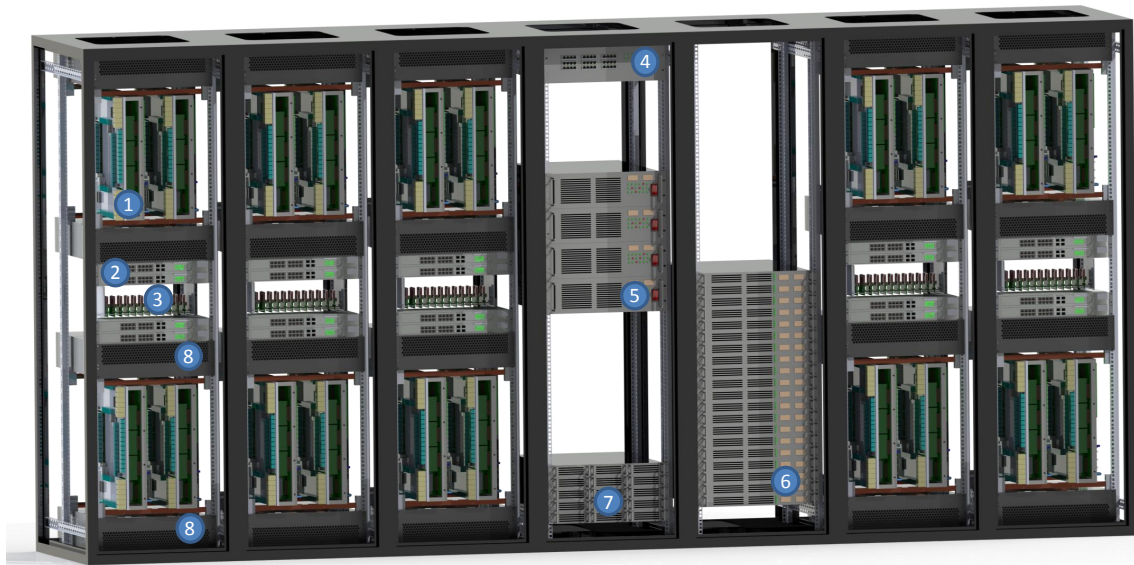
Figure 2.1.2: Rendered View of the NM-PM1 system. ① Wafer Module, ② Wafer Module network switch, ③ analog readout subsystem, ④ Top-of-Rack (ToR) 40Gbit network switch, ⑤ storage server node, ⑥ computer server node, ⑦ Wafer Module power supply, ⑧ top and bottom fan units for Wafer Module
