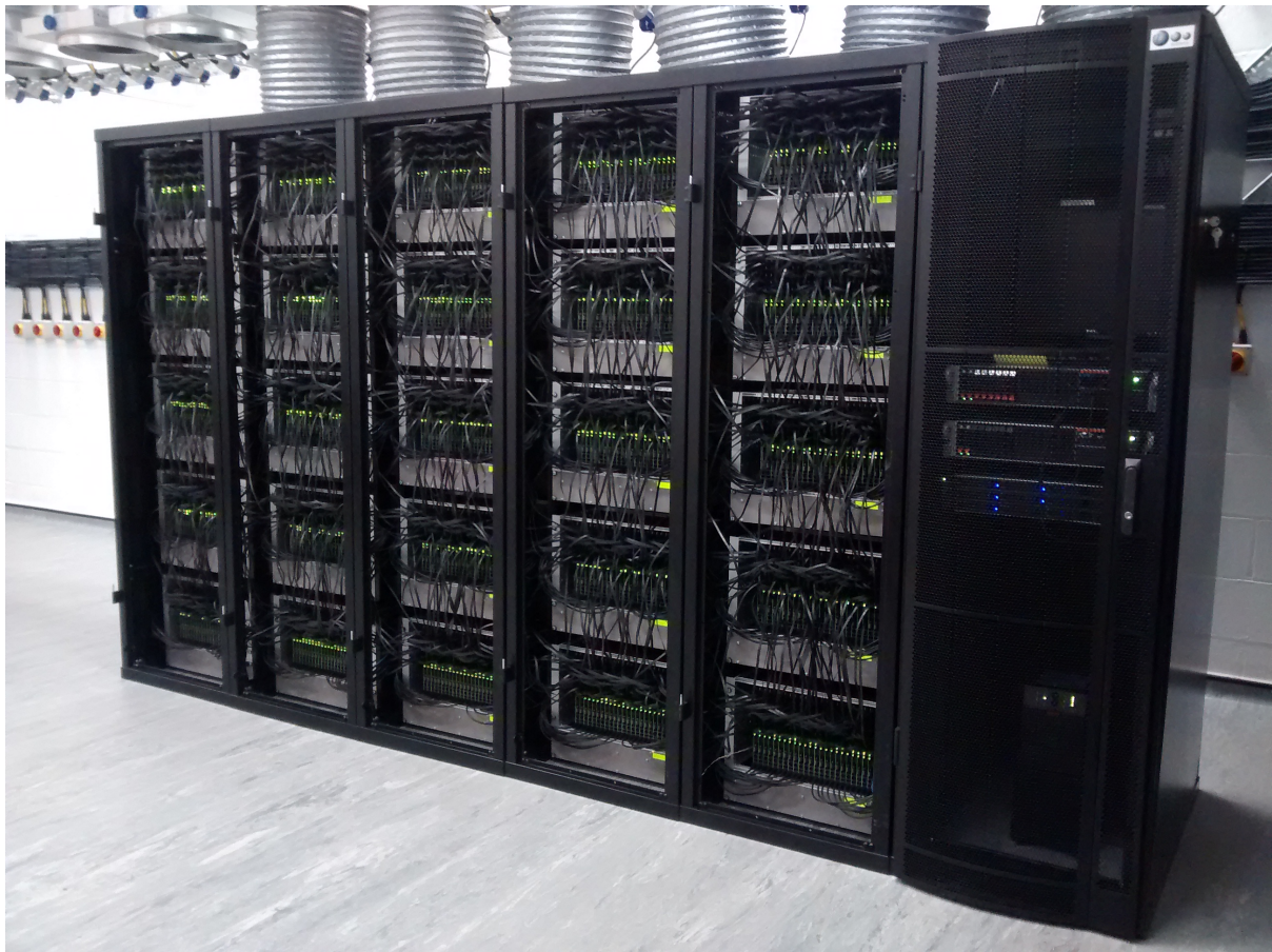
Fig. 6.1: The SpiNNaker 500,000 core system (NM-MC1) in Manchester on 25 March 2016
