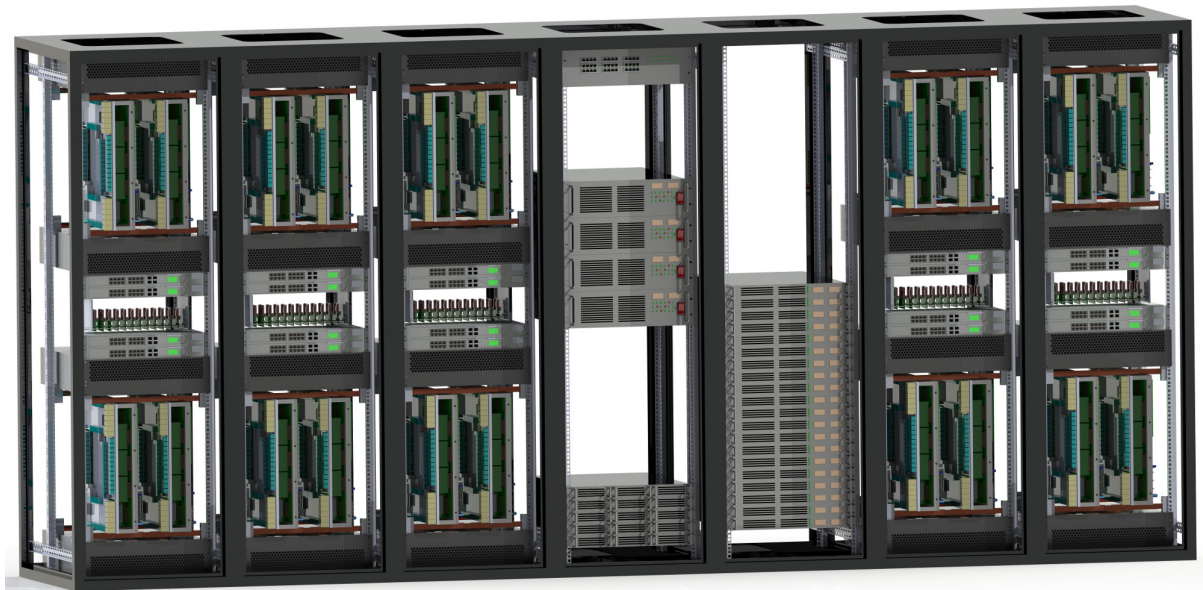
Fig. 4.2: The BrainScaleS (NM-PM-1) system: five 19-inch racks contain 20 neuromorphic wafer modules (cf. 4.1), the other two racks carry power supplies and a conventional control cluster.
