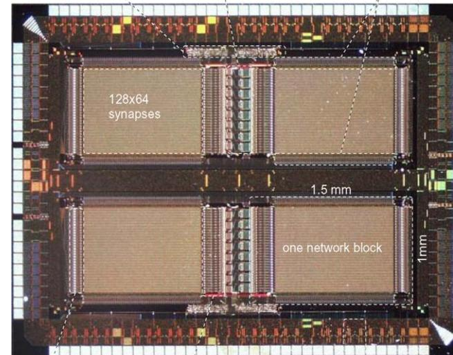
64 output neurons    analog weight storage    bidirectional LVDS IO cell
