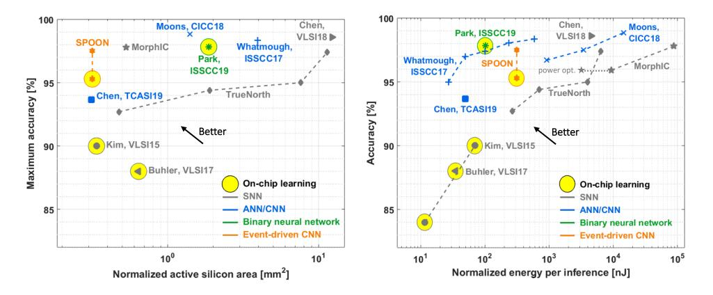
Only SPOON allows reaching the efficiency of ANN/CNN/BNN accelerators while enabling online learning with event-based sensors.
