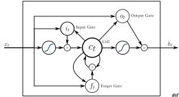
MAC accelerators for LSTM have to go back from matrix-matrix to vector-matrix and typically are limited by memory bandwidth
