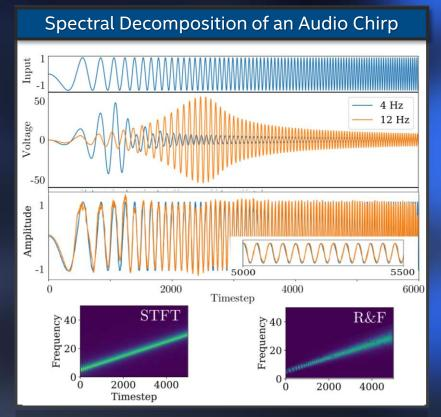
50x sparser output than conventional Short Time Fourier Transform
